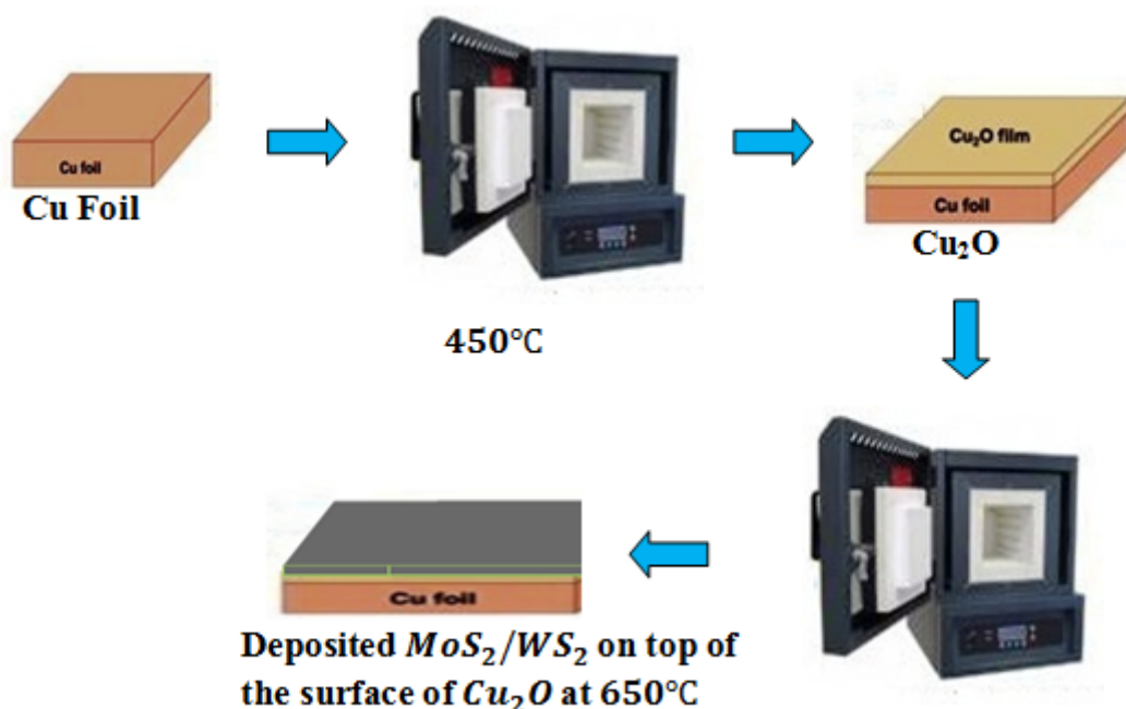
Figure 1. Schematic of a growing MoS_2/WS_2/Cu_2O film.
